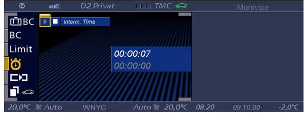
The stopwatch is ready for operation as of terminal R. A stopwatch that is running is stopped at terminal R Off and restarts at terminal R On.
